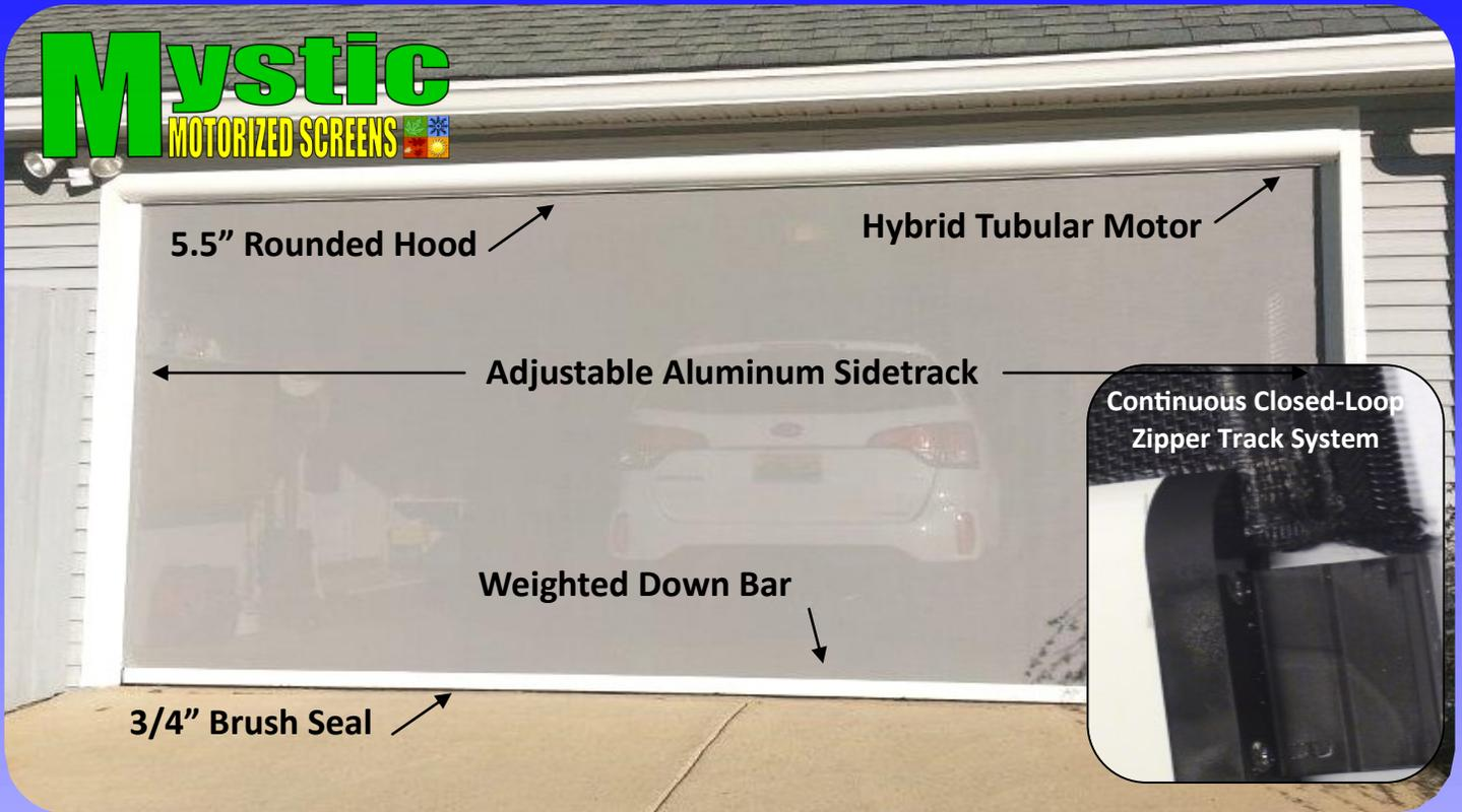
Mystic Screens use an ultra-sonic welded zipper captured in a continuous closed-loop track system. This makes Mystic better suited for use in windier conditions than competing screen systems.
